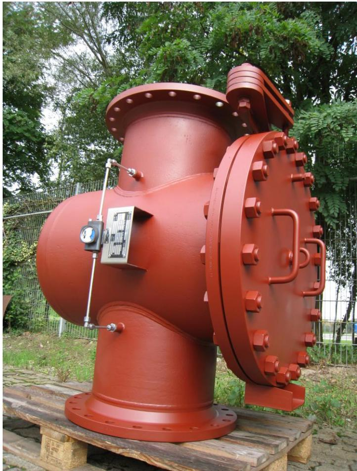
district heating network of Graz the filters are utilized in DN450 and pressure rating PN 25 with but-weld ends (SS).
